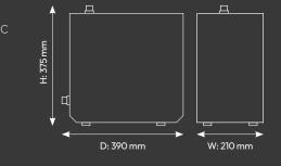
**Dimensions** (includes inlet/outlet ports)
